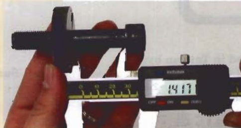
Lg measurement using SPECIAL non-counterbore GO ring gage
